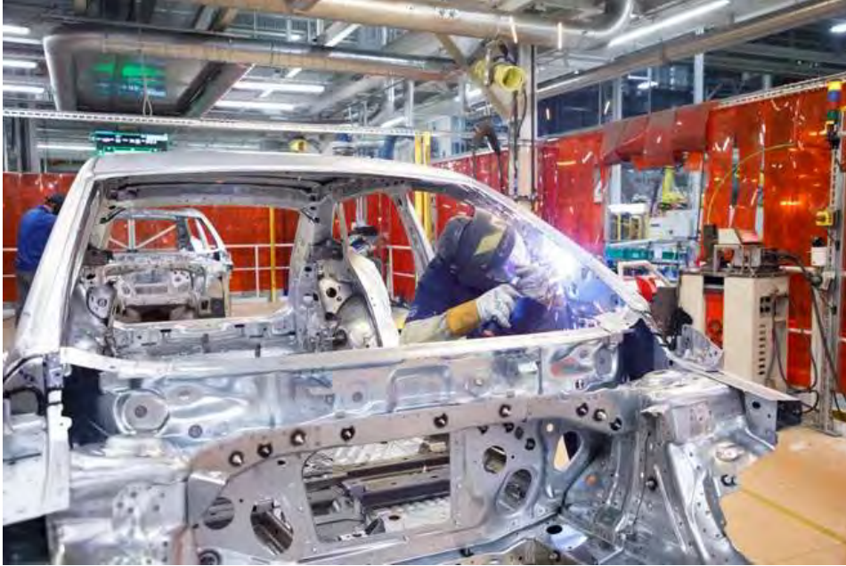
A worker welds a car body at the Volkswagen plant in Chattanooga, Tenn. Courtesy Of VW
